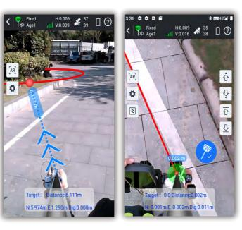
(This function only works with the receiver models that have downward-facing camera or dual-cameras)
