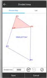
Select points to form a polygon, and directly identify the area division points for the surveyor to stake out. There is no more need for the user to guess a position to measure, and then to adjust.
