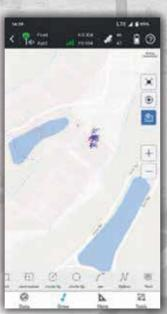
Select points to form a polygon, and directly identify the area division points for the surveyor to stake out. There is no more need for the user to guess a position to measure, and then to adjust.
