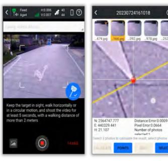
(This function only works with the receiver models that have front-facing camera or dual-cameras)
