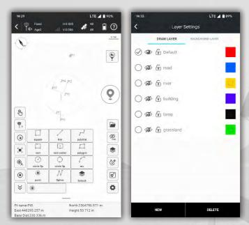
This feature allows you to draw the result map while completing point measurements.
