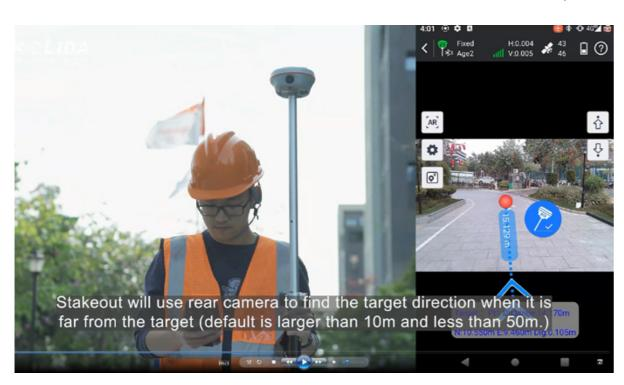
K50X allows you to implement immersive AR stakeout in any working environment. It is suitable for both non-experienced surveyor and expert to follow the visual guide to find the targets with 8MP front camera (for direction) and the 2MP camera on receiver (for precise positioning), provides up to 50% more efficiency.
