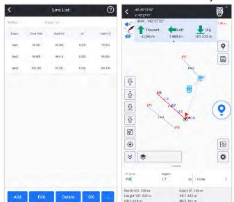
User is allowed to manually choose points from library, line will be formed by program automatically. Then user input interval distance, setout points will be calculated out and displayed on screen.
