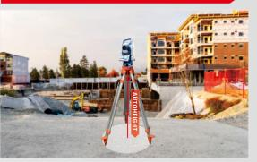
CTS-661R10 can automatically measure, read, and set the instrument height by only a simple button press. It greatly reduces errors and accelerates the setup process in job sites. The accuracy is ±1.5 mm at 1.5 m, operating range is from 0.5 m to 3 m. This feature is a national patented technology of China.
