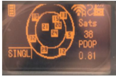
38 satellites tracked by 336 channels receiver
