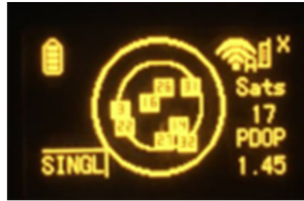
17 satellites tracked by 220 channels receiver
