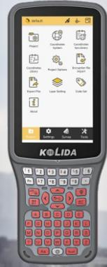
H6 is KOLIDA new generation professional Android controller. It is installed Android 8.1 OS and adopts full keypad with separate keys for 26 letters and numbers makes the input in the field more faster.
