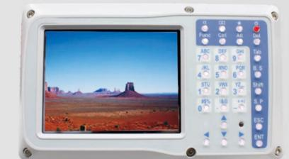
Imaging function is available on CTS-662i 3.2 mega pixel camera in front of the EDM. Capture the color images of the points you measure at anytime. Images can be saved and post-processed with relevant point information.
